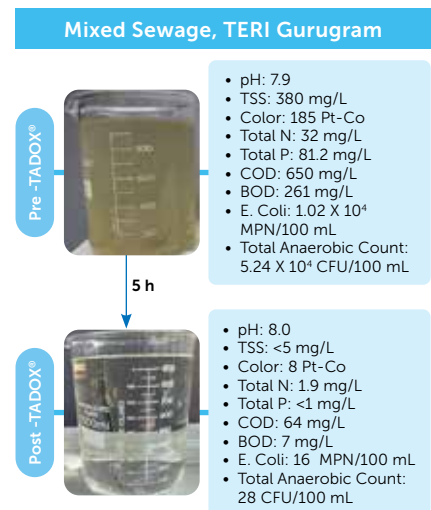
Figure 2: TADOX® treatment for mixed sewerage at 10 KLD WWTP at TERI Gurugram
